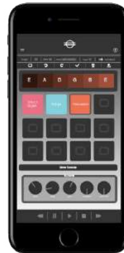
▲ Assign sound effects and patches to guitar strings to use Ludere as a MIDI Controller.
